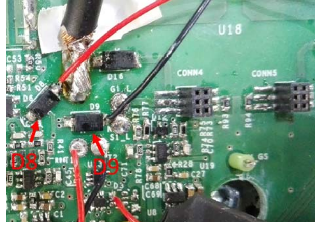
Fig. 6. Detail of the power board. The two diodes D8 and D9 are close to eachother.
