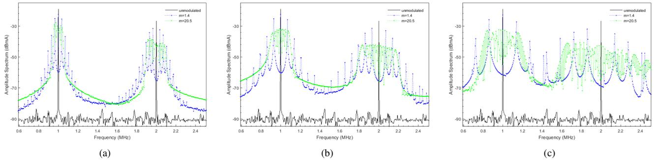
Fig. 2. Output power spectra of the converter of Fig. 1 when applying triangular-based SSC for three different values of  $\Delta f$ . (a):  $\Delta f/f_c = 0.05$ ; (b):  $\Delta f/f_c = 0.1$ ; (c):  $\Delta f/f_c = 0.2$ .
