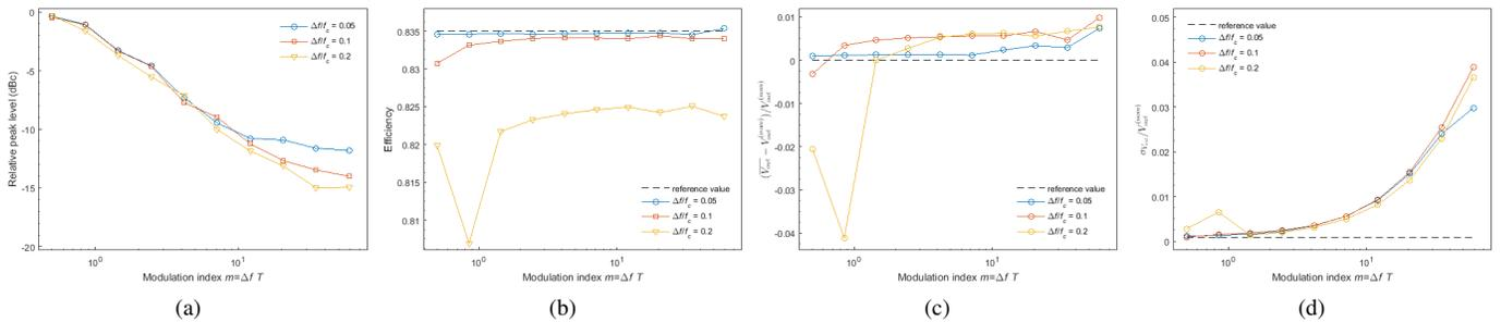
Fig. 4. Figures of merit for the class-E converter when applying triangular-based SSC for different values of  $\Delta f$  and  $m$ . (a): EMI reduction; (b): efficiency; (c): output voltage deviation; (d): output voltage ripple.
