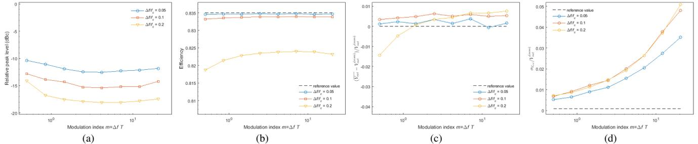
Fig. 7. Figures of merit for the class-E converter when applying chaos-based SSC for different values of  $\Delta f$  and  $m$ . (a): EMI reduction; (b): efficiency; (c): output voltage deviation; (d): ripple.
