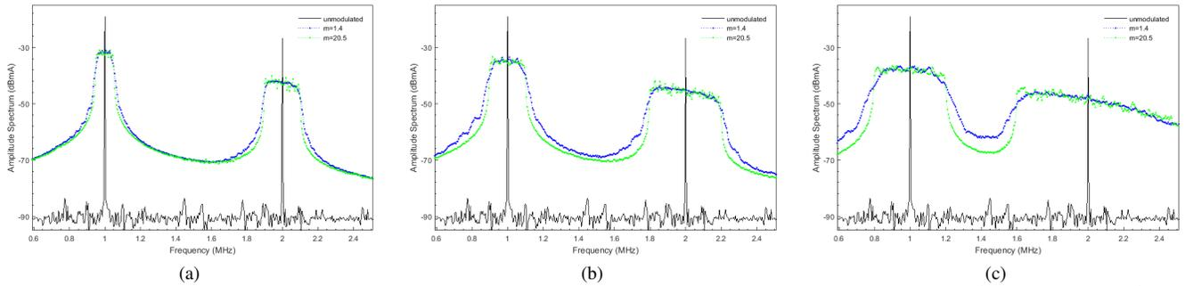
Fig. 6. Output power spectra of the converter of Fig. 1 when applying chaos-based SSC for three different values of  $\Delta f$ . (a):  $\Delta f/f_c = 0.05$ ; (b):  $\Delta f/f_c = 0.1$ ; (c):  $\Delta f/f_c = 0.2$ .
