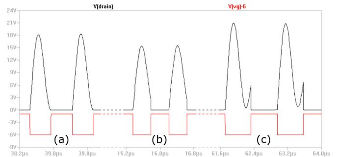
Fig. 3. When oscillating at the correct switching frequency  $f_c$  (a), the resonant converter features ZVS, i.e., the MOS is turned ON by its control clock signal (bottom plot) when  $V_{DS}(t)$  (top plot) naturally reaches zero. When applying SSC, this does not happen, and the MOS may be turned ON too early (b) or too late (c).
