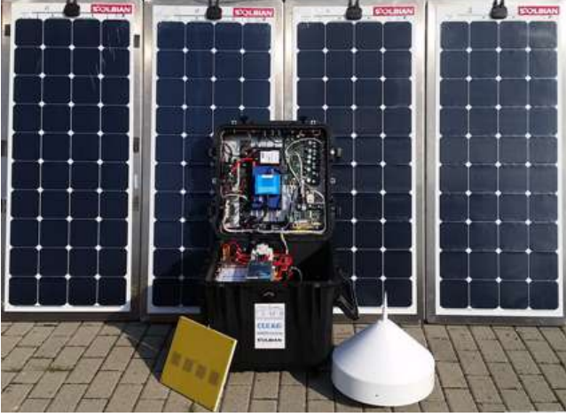
Fig. 5. Integrated prototype of the measurement station
