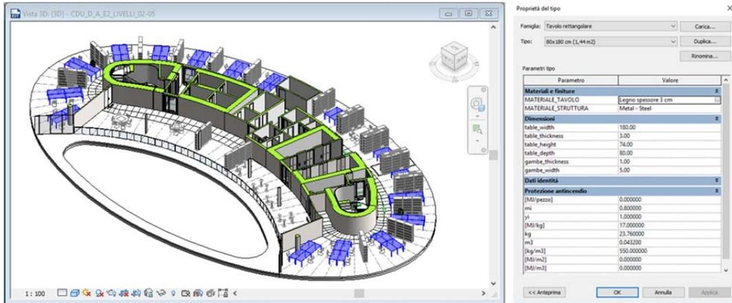
Figure 72: Desk parameters for specific fire load calculation.
