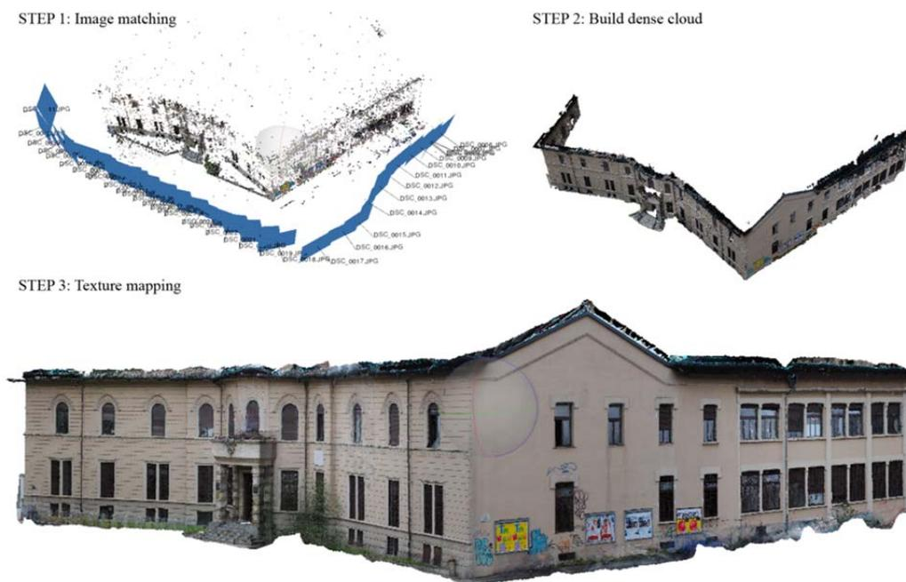
Figure 20: Point cloud realized with PhotoScan.
