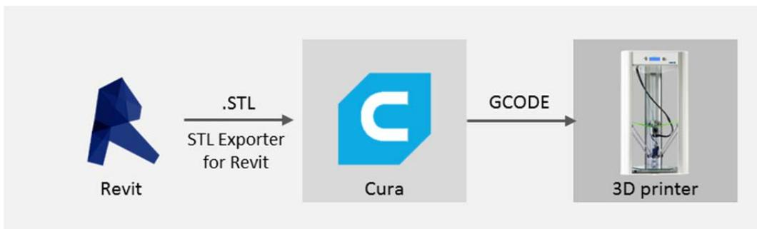
Figure 90: Revit-Cura interoperability process for 3D printing.
