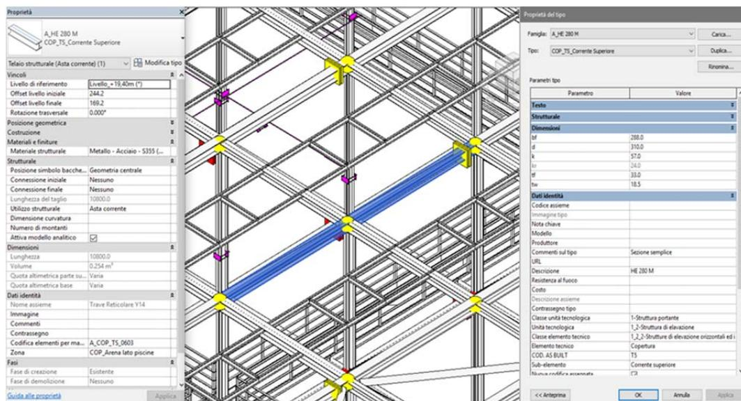
Figure 81: parametric modelling of steel structural auctions.
