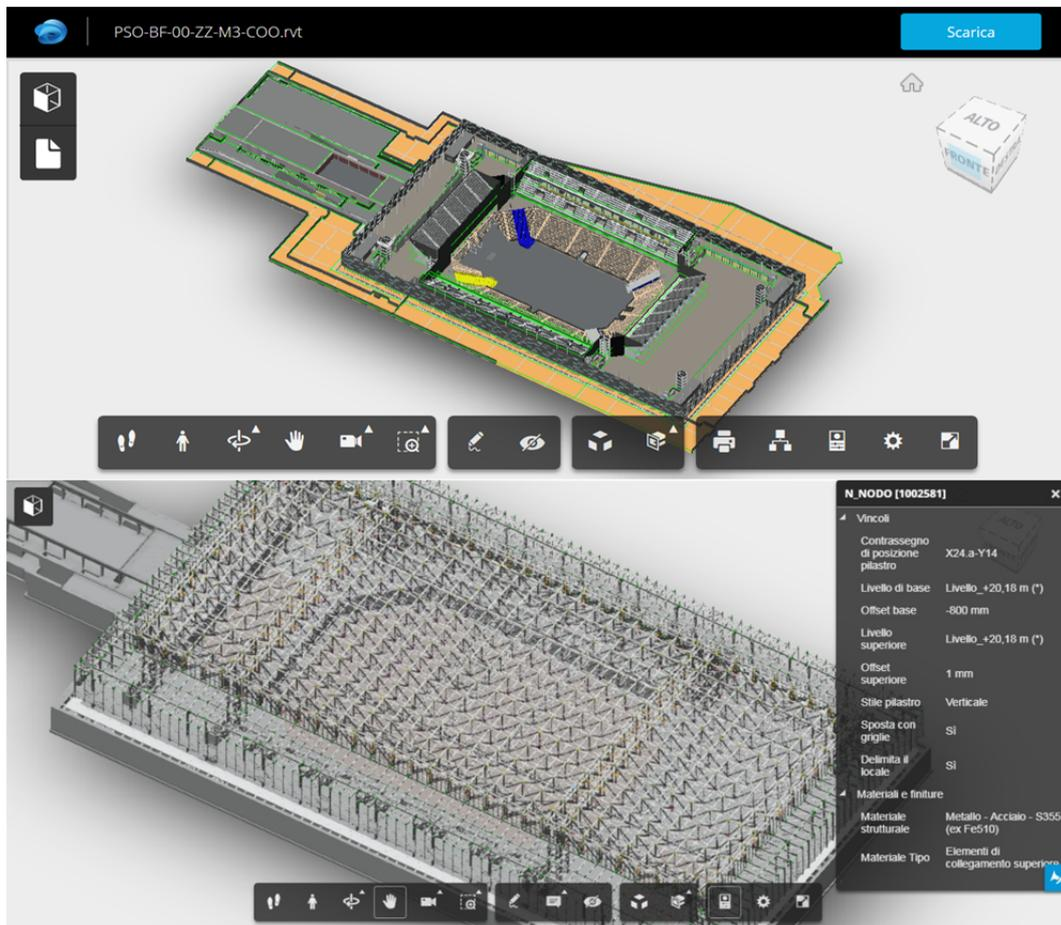
Figure 84: BIM model display through A360 viewer.
