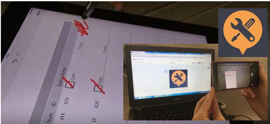
Figure 102: Marker enabling AR maintenance worksheet visualization.
