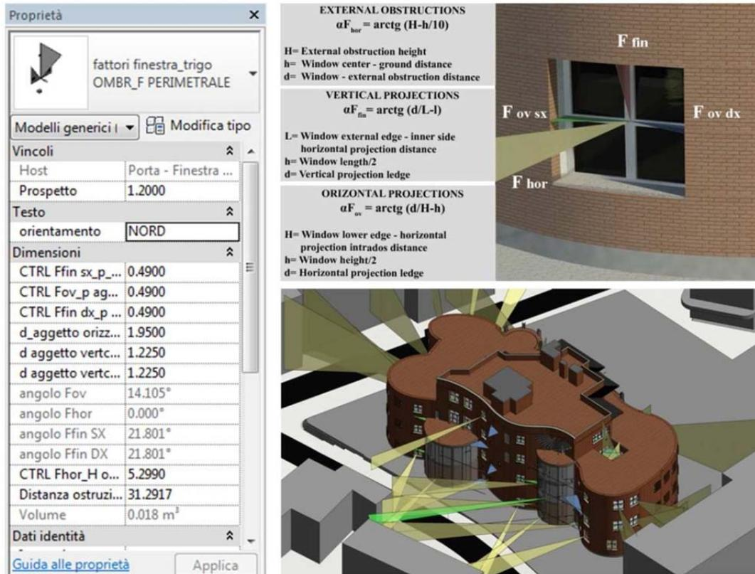
Figure 56 Surface-based Revit family for shading values calculation.
