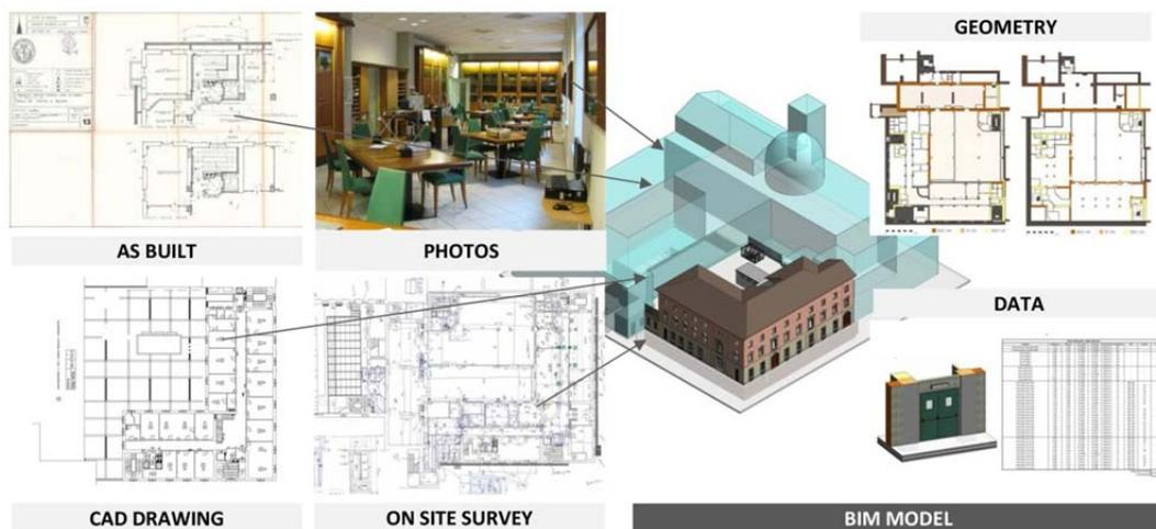
Figure 21: BIM model definition from survey and existing documentation.
