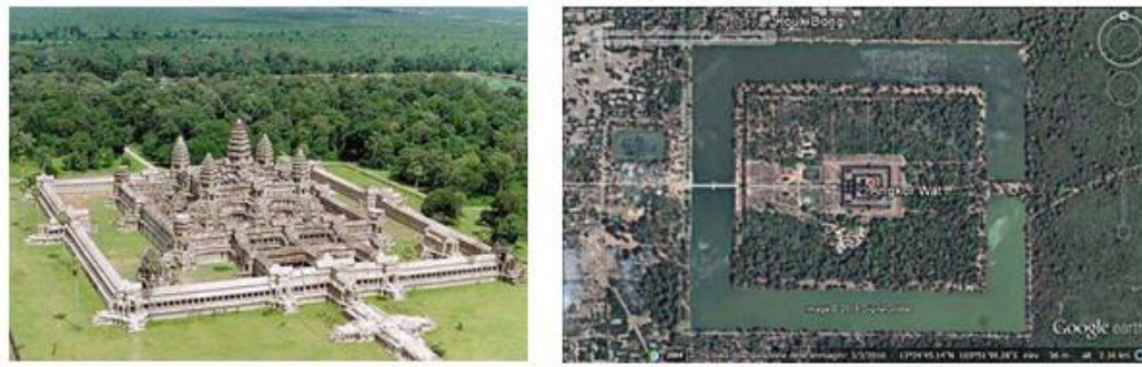
Fig. 7. On the left, aerial view of the central structure. Courtesy Shyam tnj, Wikipedia. On the right, the Angkor Wat surrounded by a moat used for helping stabilize the temple's foundation [31]. Courtesy: Google Earth.
