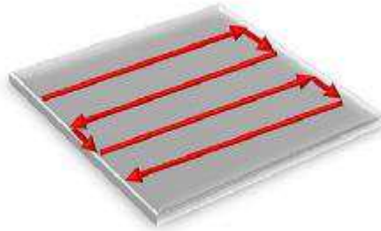
Figure 25: Illustration view of the zig-zag deposition strategy used for DED process (the read arrows indicate the laser tracks) [56].
