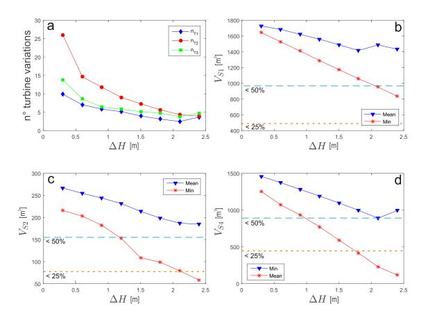
Figure 8. (a) Number of flow rate variations in a day for turbines T1, T2 and T3. (b)-(d) Minimum and mean water volume stored in tanks S1, S2 and S4 for different  $\Delta H$ . The dashed and dotted lines mark the 50% and 25% of the total tank capacity, respectively.
