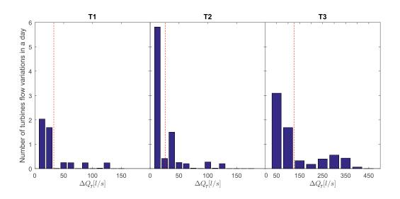
Figure 5. Daily number of flow rate variations with magnitude  $\Delta Q_T$  for turbines T1, T2 and T3. The dashed line indicates the average magnitude of  $\Delta Q_T$ .
