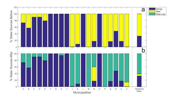
Figure 6. Composition of the water sources supplying each local network (a) without water from WPP and (b) with the water from WPP. The last bar on the right reports the mean composition in the entire valley.
