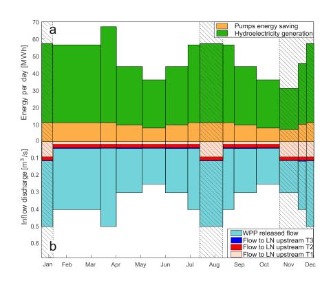
Figure 7. (a) Daily energy saving and hydropower generation over a typical year. (b) Released discharge from the WPP, flow delivered to the local networks upstream T1, T2 and T3. The hatched areas highlight touristic seasons.
