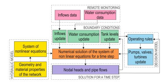
Figure 2. Scheme of the numerical model developed to simulate the operation of the new WSS.
