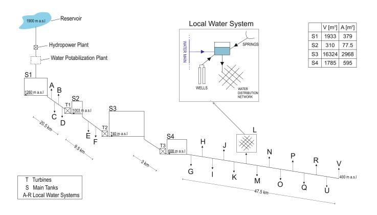
Figure 1. Scheme of the WSS. The capital letters (A,B, ... V) indicate the local water networks. The inset shows a typical local water system with a storage tank supplied by mountain springs, local wells and by the new water main.
