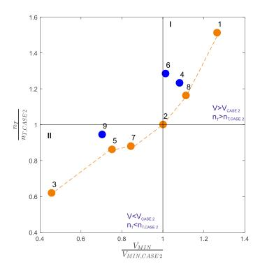
Figure 9. Number of turbine operations against minimum water storage in tanks for different combinations of  $\Delta H_1$ ,  $\Delta H_2$ ,  $\Delta H_4$ , in relation to the case of Table 1. The points lying on the Pareto front (dashed line) are the nondominated solutions. Notice that scenario 2 corresponds to Table 1
