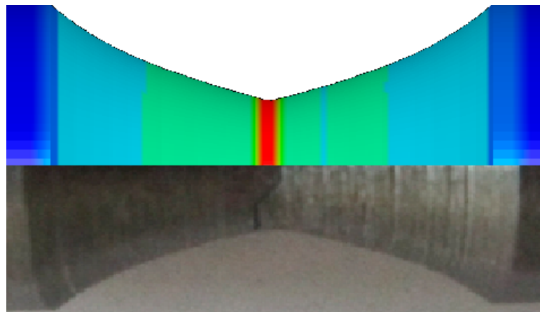
Figure 13. A comparison between the profiles of specimen measured from numerical simulation and quasi-static test.
