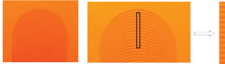
Figure 2. Example of instantaneous fringes pattern generated in the oil film and selected area.
