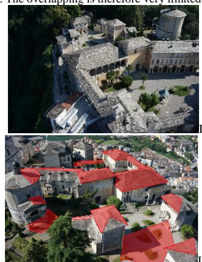
Figure 7. Example of the same area acquired in near strips, with opposite flying directions; the overlapping areas are underlined (in red in II).
