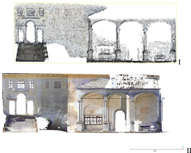
Figure 17. The compared point clouds segments: from VisualSfM (I) and from TLS survey (II).
