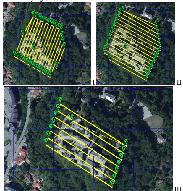
Figure 10. Flight plan with Mission planner. Nadir flights (I and II), and the oblique one (III).
