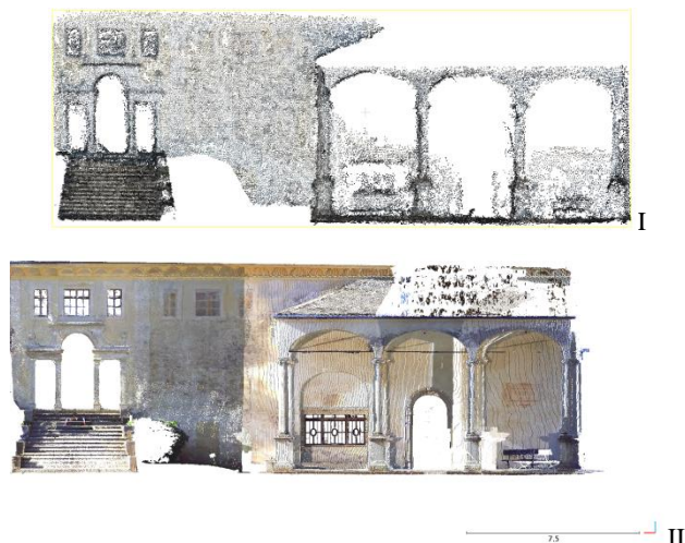
Figure 17. The compared point clouds segments: from VisualSfM (I) and from TLS survey (II).
