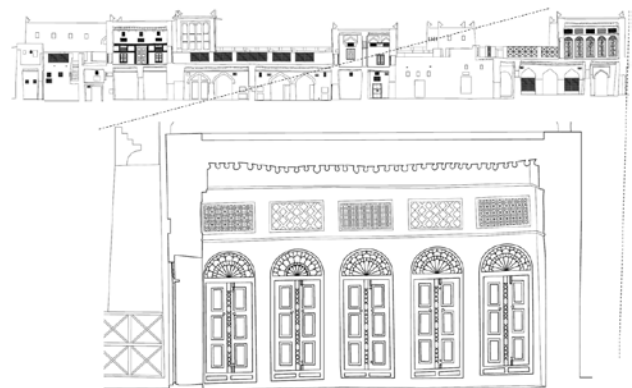
Figure 10 Example of cross section and local detail that shows the geometric irregularity of the building.
