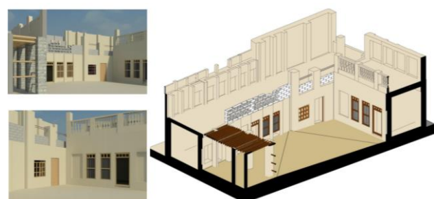
Figure 13 BIM model of the Aljazzaf house developed from the consolidated pointcloud and render samples generated from the BIM model. Software employed Autodesk Revit 2016. Images source Authors and Marwa Reyadh Alarayedh.
