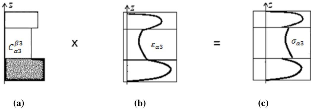
**Fig. 3** - Typical thickness-wise distributions of (a) transverse shear elastic stiffness coefficients, (b) transverse shear strains, and (c) transverse shear stresses, in a laminated structures if the in-plane displacements are assumed to be at least  $C^1$ -continuous functions of the  $z$ -coordinate.
