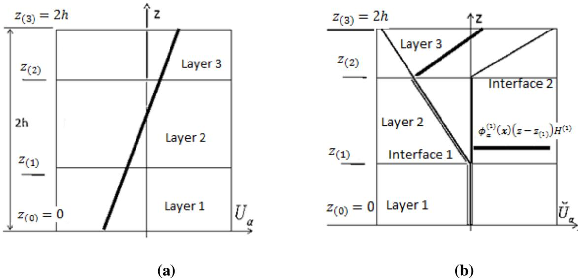
**Fig. 5** - (a) Global ESL FSDT and (b) local enrichment in the Di Sciuva's FSDZT.
