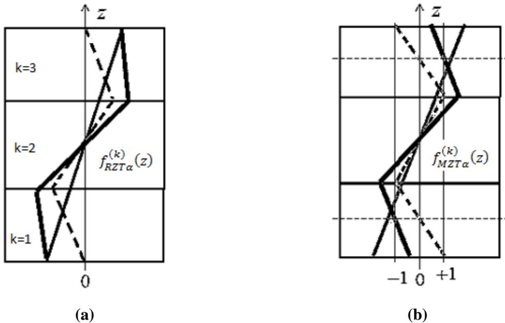
**Fig. 8** – Kinematics of (a) RZT and (b) MZT. ( ——— ) global contribution (ESL FSDT), ( - - - ) local contribution (zigzag function), ( ——— ) resulting kinematics, for a three-layer symmetric laminate.
