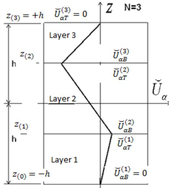
**Fig. 7** – Refined Zigzag function for a three-layer laminate.
