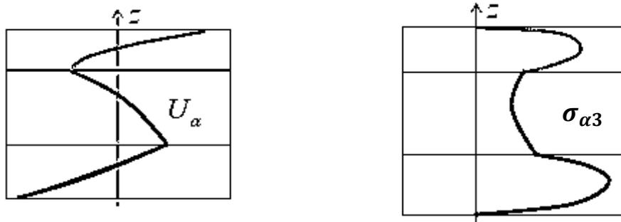
**Fig. 2** - Thickness-wise distribution of the (a) in-plane displacements and (b) transverse shear stresses. Both the distributions are of the zigzag type, that is, their derivative along  $z$  is discontinuous at the interface (zigzag behavior).
