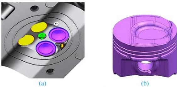
Figure 1. Combustion chamber of the developed NG engine: (a) cylinder head; (b) piston
