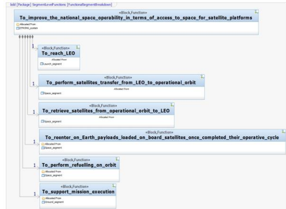
Fig. 7. Block Definition Diagram for segment functional breakdown of STRONG system
