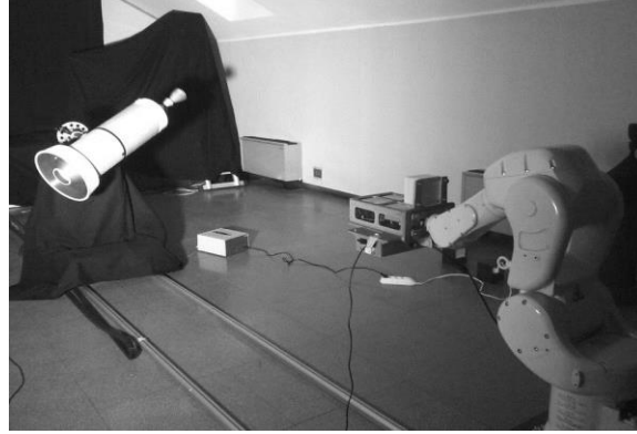
Fig. 11: The CADETLab Environment. The IR camera is mounted on an articulated robotic arm
