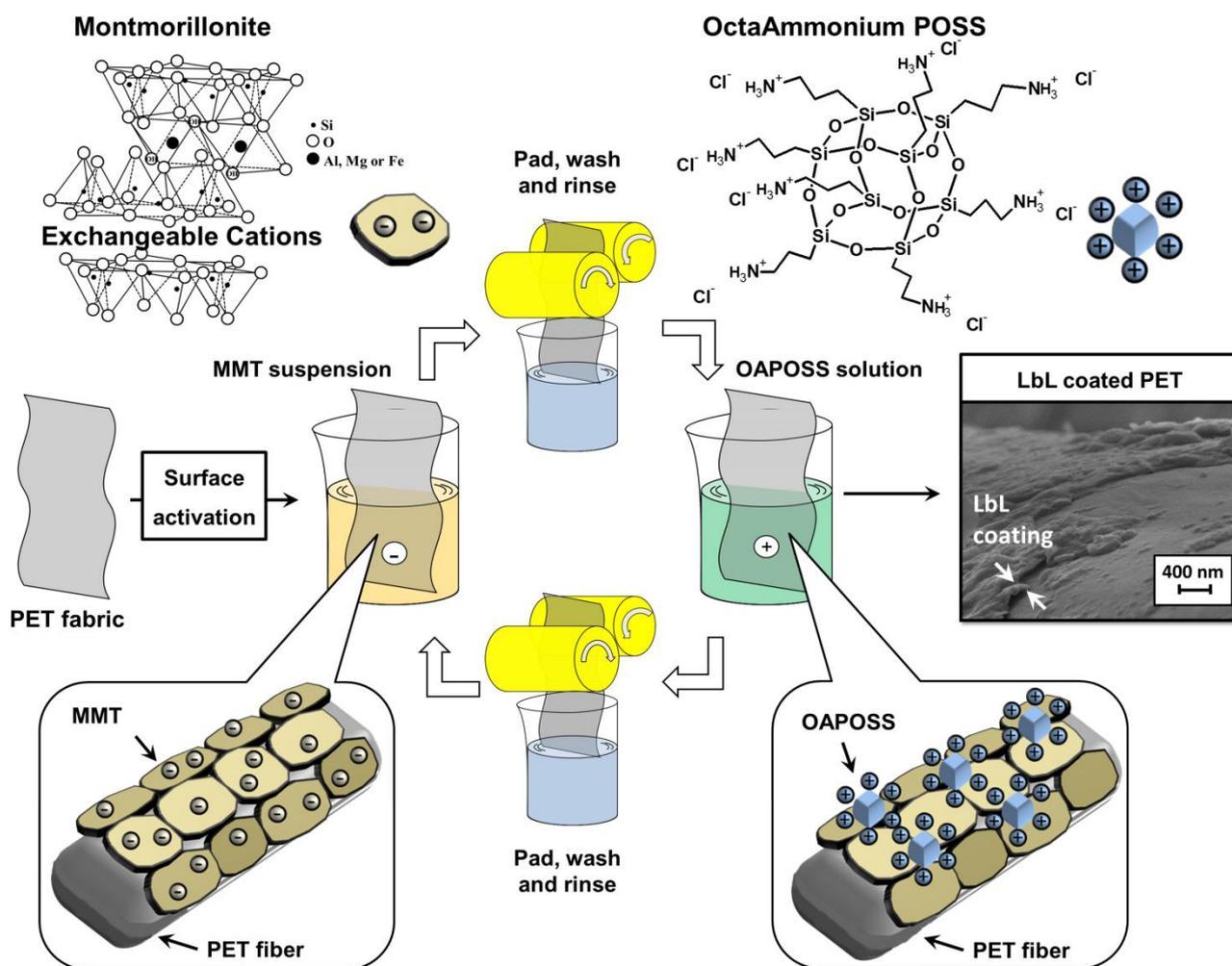
**Figure 1.** Schematic representation of the LbL process adopted in the present study. The PET fabric is primed by a branched poly(ethylene imine) - B-PEI - and then alternatively dipped in MMT suspension (negative) and OAPOSS solution (positive) until 5 BL are reached.
