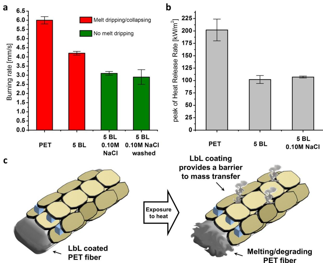
**Figure 4.** Main parameters of flammability and cone calorimetry tests: a) burning rates and occurrence of melt-dripping phenomenon, b) peak of Heat Release rate and c) schematization of the coating flame retardant mechanism.
