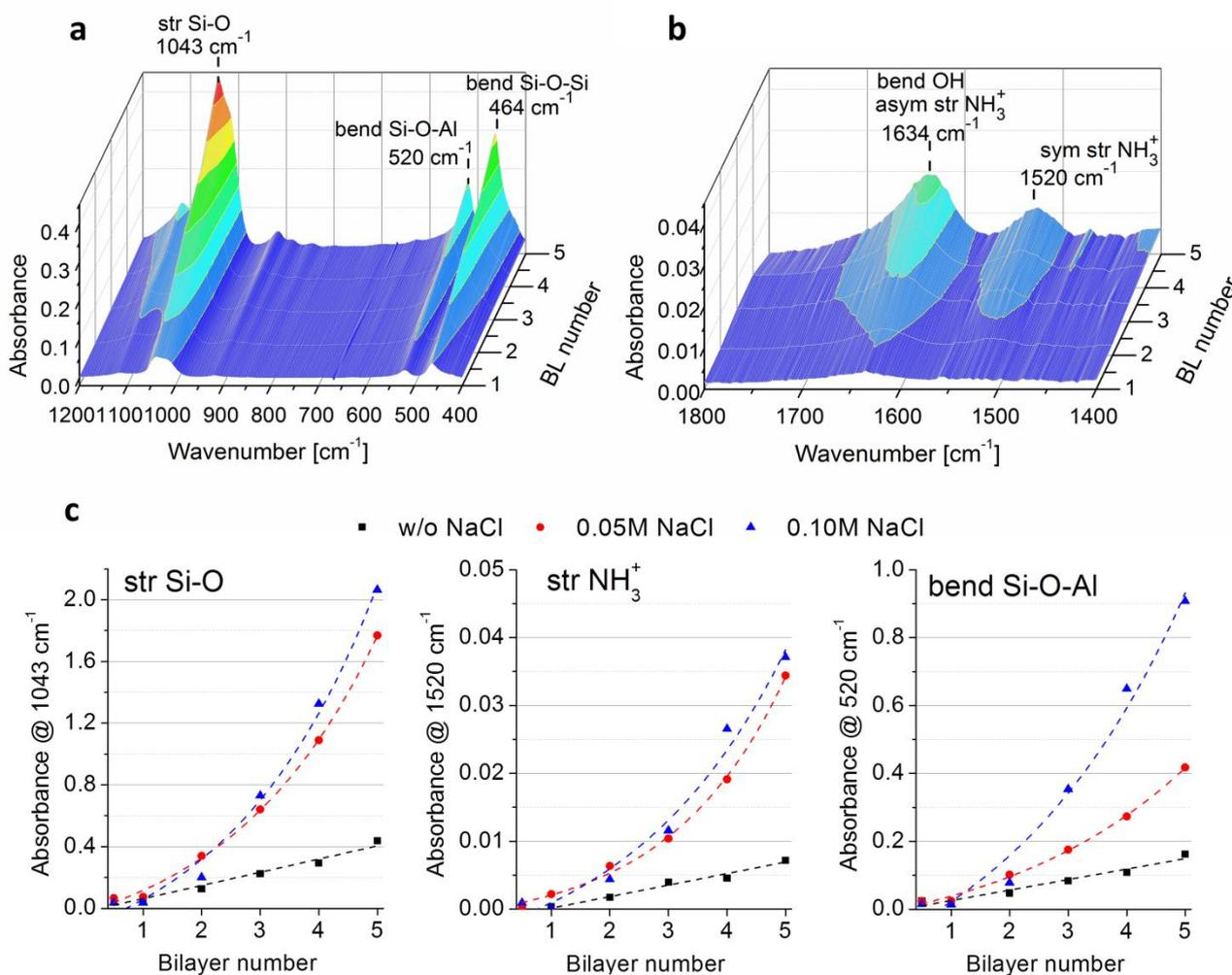
**Figure 2.** IR characterization of LbL assembly: 3D plot absorptions in the 1800-1400 (a) and 1200-400  $\text{cm}^{-1}$  (b) of LbL assembled OAPOSS/MMT unmodified ionic strength and signal intensity of 1043, 1520 and 520  $\text{cm}^{-1}$  as a function of BL number at different ionic strengths (c).
