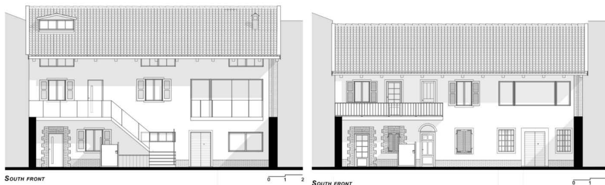
Fig. 2. Architectural design of south façade in the high investment scenario (on the left) and in the low investment one (on the right).
