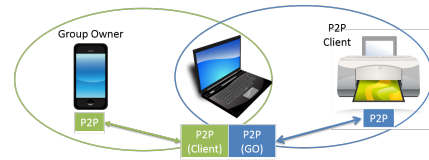
Fig. 1: Communication between two Wi-Fi Direct groups.
