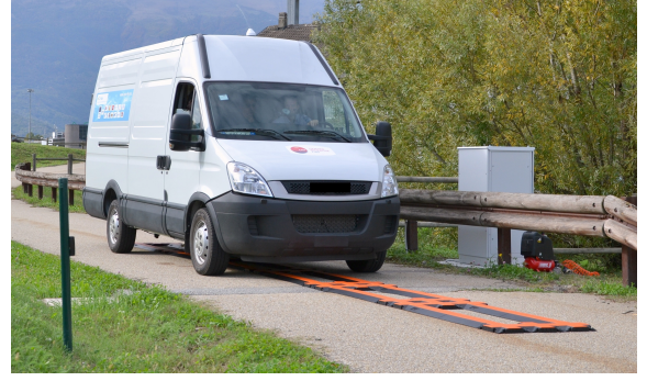
Fig. 9: First prototype of a dynamic IPT system for a light commercial vehicle within the eCo-FEV project (Italy).
