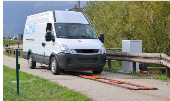
Fig. 9: First prototype of a dynamic IPT system for a light commercial vehicle within the eCo-FEV project (Italy).
