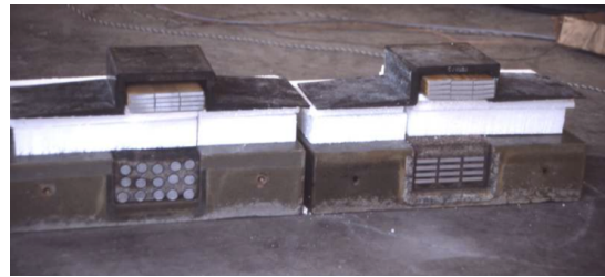
Fig. 3: Cross-section of the buried transmitter and the on board receiver of the PATH prototype [12] (reprinted by permission).
