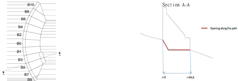
Figure 10: Path of the calculation of the opening at dam/foundation interface
