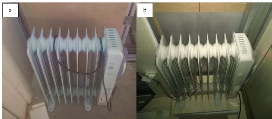
Fig. 5. (a) Configuration A (bulk wall); (b) Configuration B (wall coated with low-E paint)
