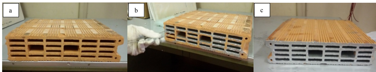
Fig. 1. (a) Rough brick used as reference case (brick A); (b) Coating phase (c) Brick with Low-E coating (brick B).
