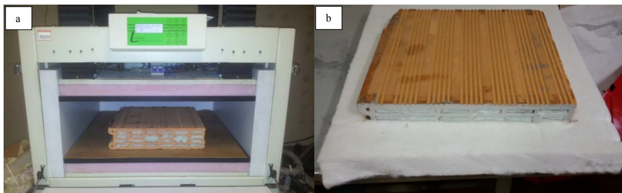
Fig. 2. (a) Brick placed in GHFM apparatus. (b) Insulation ring surrounding the brick specimen;
