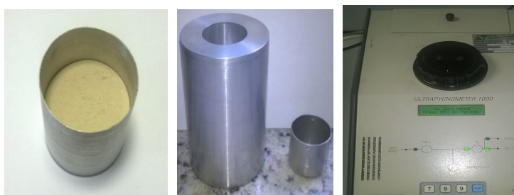
Fig. 8.11 - Dried silty sample (left, middle) and gas ultra-pycnometer 1000 (right).
