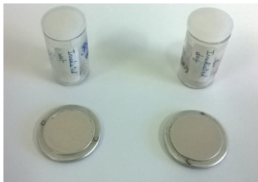
Fig. 8.18 - Dry irradiated and wet irradiated Stava tailings into sample-holder before XRD analyses.
