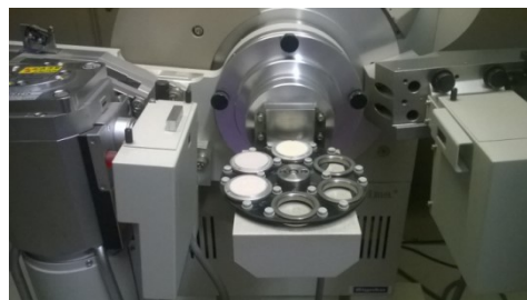
Fig. 8.17 - Working principle (a) and XRD diffractometer used at CDTN laboratories (b).
