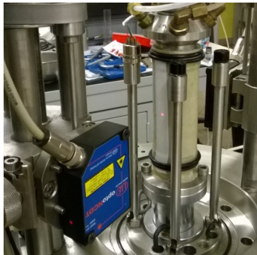
Fig. 6.13 - (a) Schematic view Laser device (Romero, 1999) and (b) picture of the laser set-up with specimen.
