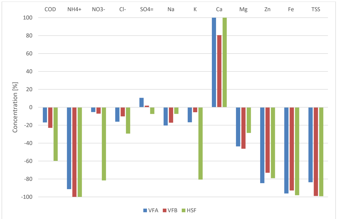
Figure 3 Main water parameters removal percentage (compared to inlet wastewater) for each CWs tank (VFA, VFB and HF).
