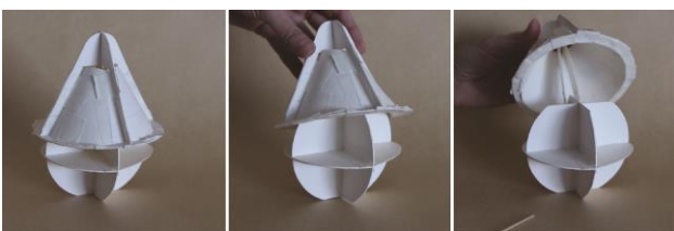
Figure 7 | Second paper prototype. The hat has the shape of a cone, rounded on top. The two elements are joint by providing the hat with two axes joint to the structure of the body through a pivot.
