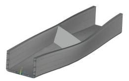
(b) ANS3D deformed mesh, Max. displacement=0.99 mm (DOF=762264)
