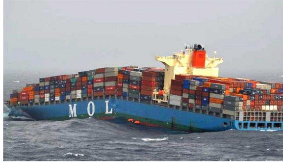
Figure 1.1 A container ship failure under global loads
