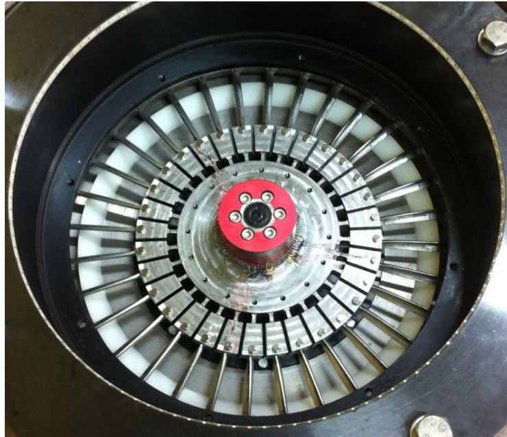
Fig. 6.5 The dummy disk 2 within the spinning test rig.
