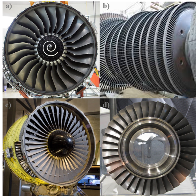
Fig. 2.2 Examples of cyclic symmetric structures.
