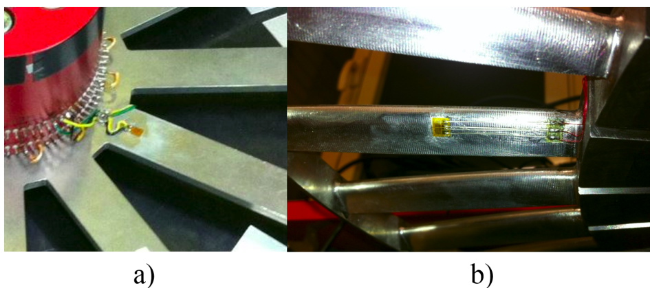
Fig. 6.8 Strain gauge at the blade root of the dummy disk 1 a), strain gauge at the back of the airfoil of a dummy disk 2 blade b).
