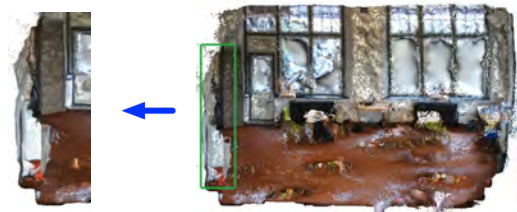
Figure 11. The area with green rectangle in the mesh model is a locker, which is a concave space from the bottom view.
