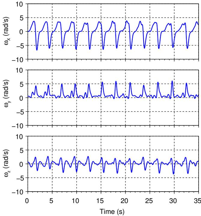
Fig. 6. Angular velocity traces after the rotation to minimize the cumulative angle on  $x$  and  $z$  axes.
