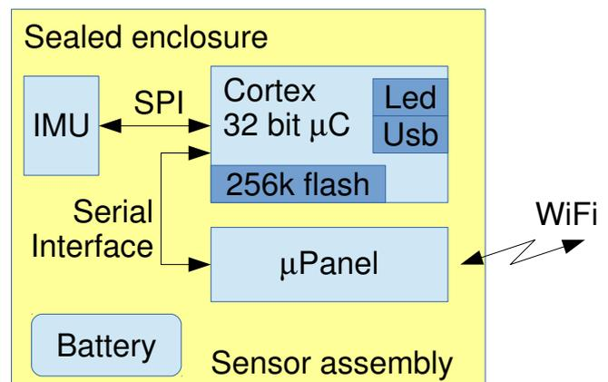
Fig. 1. Block diagram of the proposed sensor assembly.
