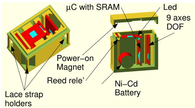
Fig. 3. The sensor assembly: the sealed box which contains the IMU, the Teensyduino microcontroller, the  $\mu$ Panel wireless board, the power on reed relé and the magnet, the NiCd battery and the led for the user feedback.
