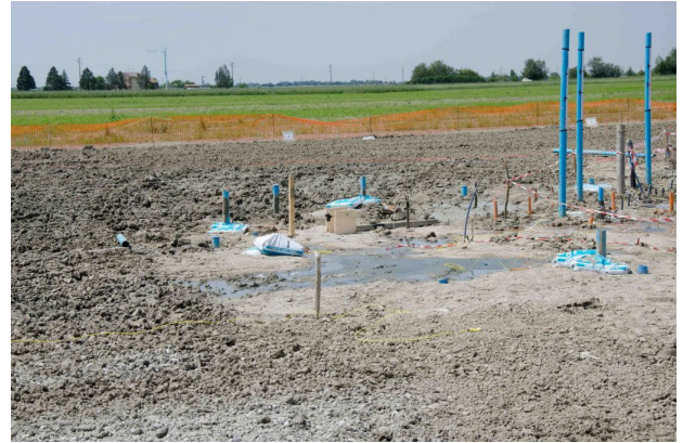
Figure 9. Blast-induced sand boils after the first detonation.
