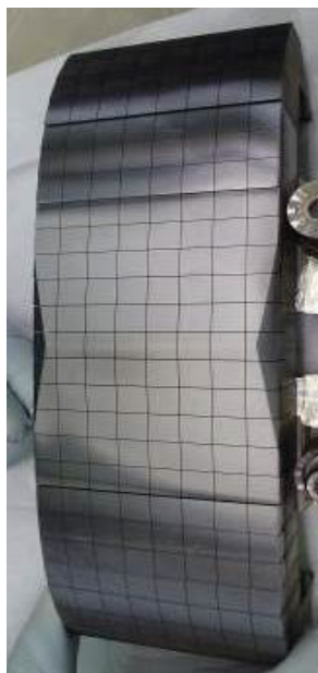
Figure 3. Left: castellated beryllium limiter tile from JET-ILW; right: deposition profiles of deuterium inside the castellated groove of a Be limiter; insert: side of a sectioned tile.
