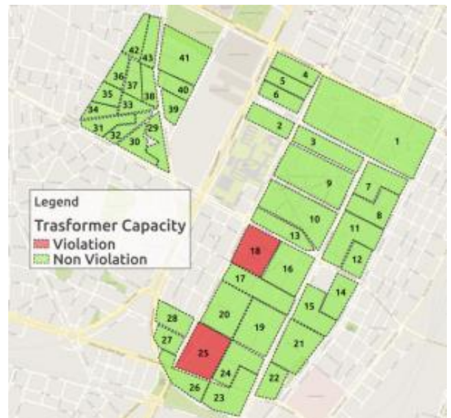
Figure 6. Transformer violation capacity map
