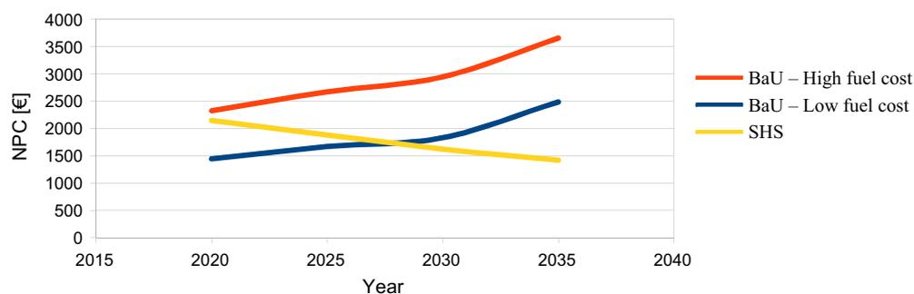
**Fig. 2.** Evolutionary NPC of the SHS technology versus the BaU Scenario. Low fuel cost: €15/M on the short term going up to €20/M on the long term. High fuel cost: €25/M on the short term going up to €30/M on the long term.
