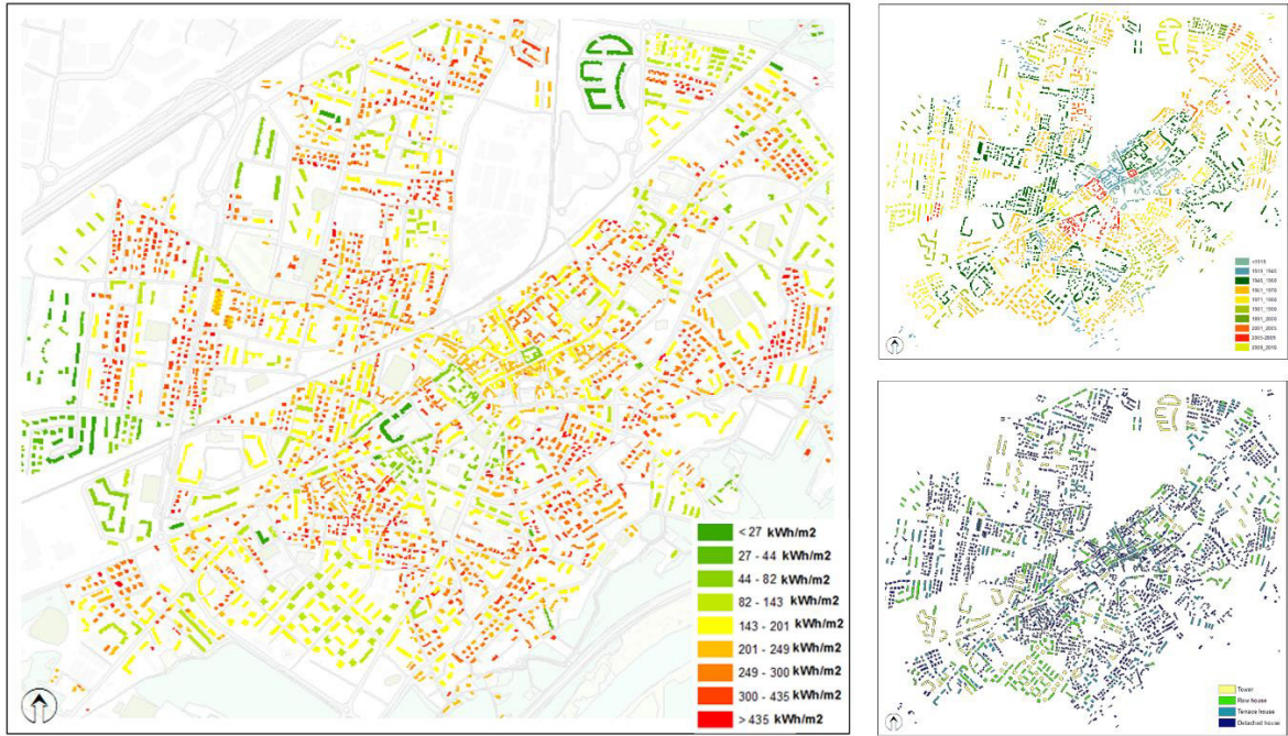
Fig. 2. (a) The final energy consumptions for heating (kWh/m 2 y) (left); (b) An image representing the prevailing age for each census area (up right) and the Surface ratio to the volume (down right).
