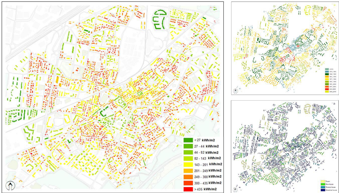
Fig. 2(a) shows the final energy consumptions map for heating (kWh/m 2 y) as well as an image representing the prevailing age of buildings for each census area and the buildings' typology and archetypes (see Fig. 3.(b)).
