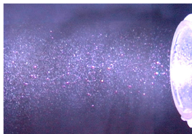
Fig. 9. Dispersed flow at the pipe outlet; nozzle type 1.25 at 2 barg.
