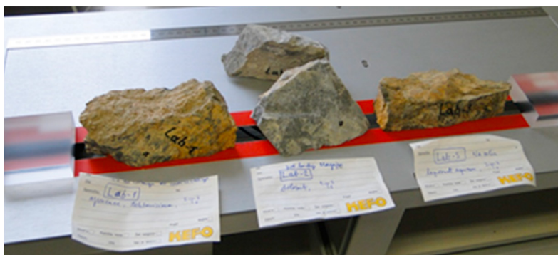
Fig. 3 Scanning of some rock samples (limestone, dolomite, marly limestone) with the TCS meter.
