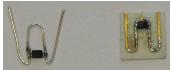
FIGURE 7 Two implementations of the “w-shaped” transponder, manufactured with a bent copper wire (left) and with a printed wire (right)
