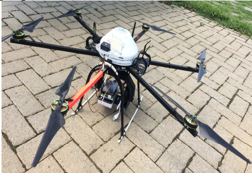
Figure 1. The employed multi-rotor platform used for the image acquisition
