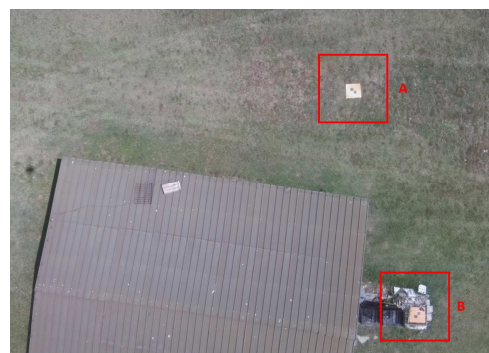
Figure 6. Marker placed on the ground (a) and on a structure in elevation (b).
