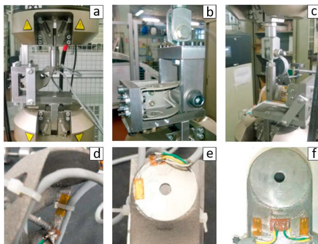
Fig. 5: First row: experimental set-up for the component static strength test: (a) load case 1; (b) load case 2; (c) load case 3. Second row: locations of the strain gauges for load case 1 (d), (e) and for load Case 2 and 3 (f).
