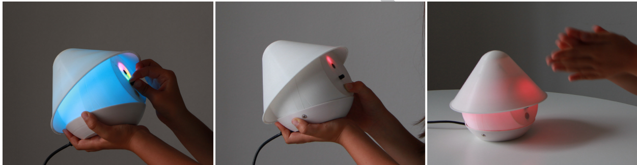
8. Fig. 9. From the left: colour selection (A), sound recording (B), and scared status (C).
