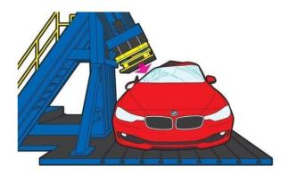
Figure 3.9: Schematic of roof crush test
