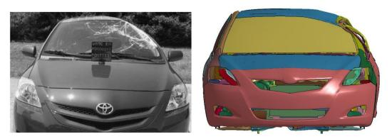
Figure 6.45: Comparison of real and FEM roof crush test
