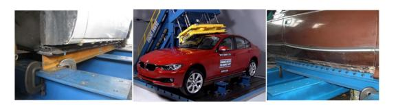
Figure 6.32: FMVSS 216 experimental test configuration [2]
