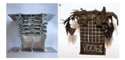
Figure 3.13: Comparison of metallic specimen folding and composite specimen fracture [4]
