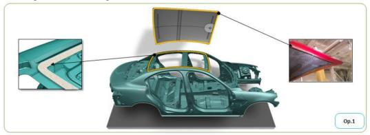
Figure 7.4. First step of pre-assembly of roof panel [1]
