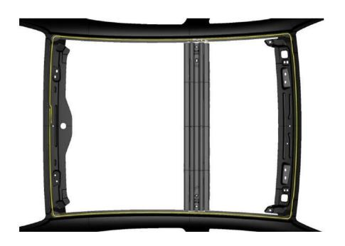
Figure 7.2. Adhesive path on the roof panel [1]
