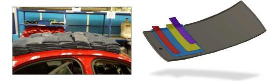
Figure 7.1: Roof fiber lay-up orientation [1]
