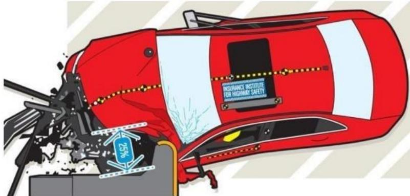
Figure 3.5: Schematic of 20% frontal offset crash
