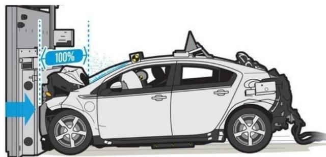
Figure 3.4: Schematic of full frontal crash test
