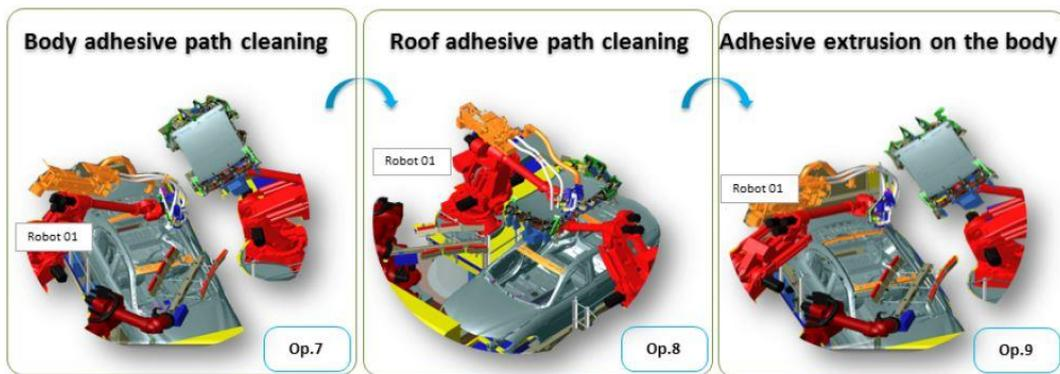
Figure 7.6. Automated assembly first steps [1]
