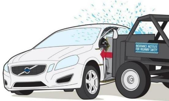
Figure 3.7: Schematic of side crash test
