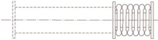
Figure 3.10: Axial collapse mode [1]
