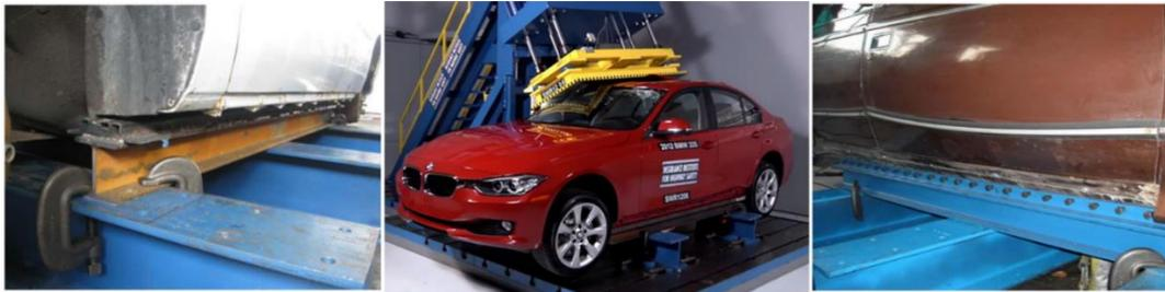
Figure 6.32: FMVSS 216 experimental test configuration [2]
