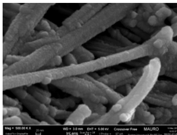
Fig. 2. (a) micrograph of thermally treated sepiolite; (b) FE-SEM micrograph of thermally treated leached sepiolite; (c) FE-SEM micrograph of zinc doped sepiolite.
