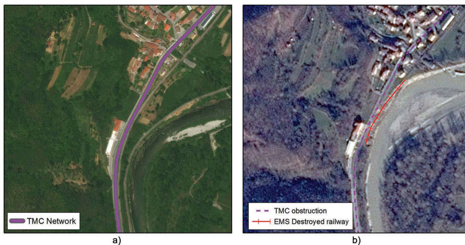
Figure 14. Damages to the transportation network. (a) shows the pre-event situation. (b) shows how EMS-Mapping reported damages only to the railway network while TMC reported an obstruction event to the nearby road too.
